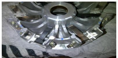
The 3 stock and 3 adjustable weights are alternating. The 3 stock are 120 degrees apart, as are the 3 new ones. – Every second one is replaced. <u>THIS IS THE ONLY CONFIGURATION THAT 3 WEIGHTS CAN</u> <u>BE REPLACED.</u>
