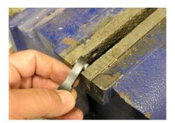
1) Push and hold the rivet ALL the way through the hole in the flyweight. (**remember to keep all rivets same direction**)
